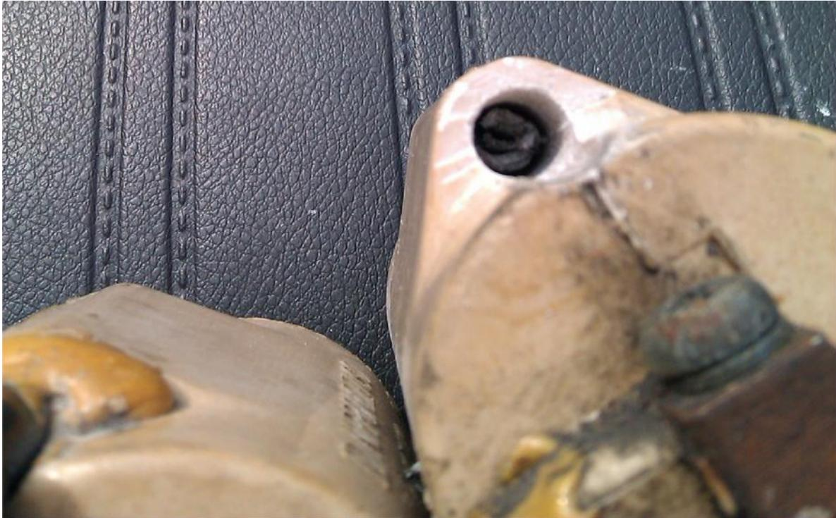
***All leads removed and housings thoroughly cleaned to ensure good electrical contact***
